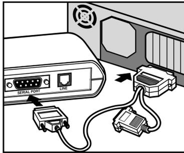
**Note:** Connect the male end of the RS-232 cable to the modem's serial port and the female end to your computer. Choose suitable 9-pin or 25-pin female connector according to your computer's serial port.
