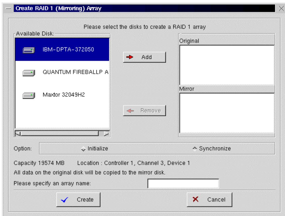
2 All the detected available disks on your system are listed in the **Available Disk** list box. You can specify the original disk and the mirror disk by selecting the disk and clicking **Add** button to add it to the **Original** box and **Mirror** box.
