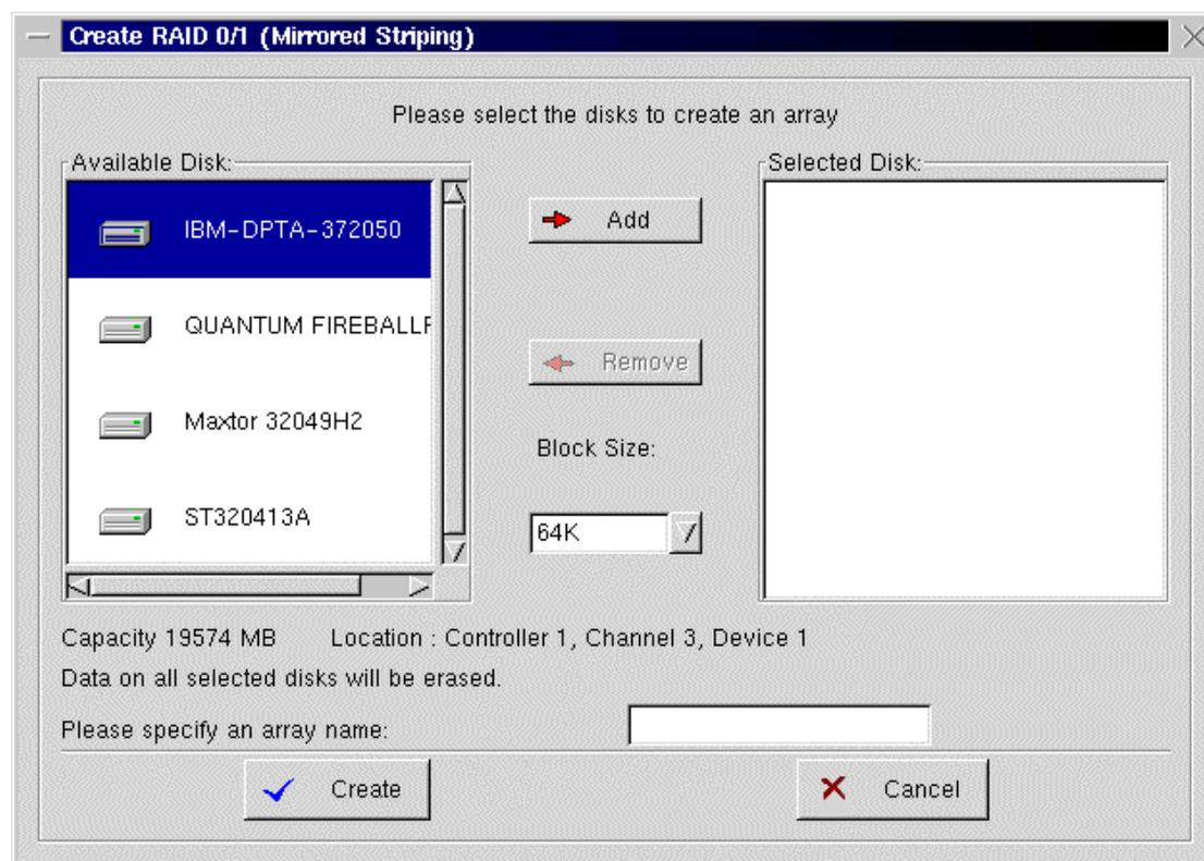
**Note:** You must attach at least four hard disks to the controller to create a RAID 0/1 array.
