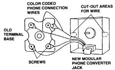
A modular jack converter (not included) is required, entailing some rewiring (namely, making color-coded connections).
