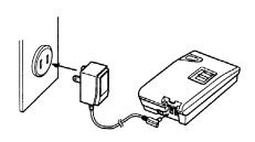
Connect the plug at the end of the AC adaptor to a standard 120V AC outlet and the other end to the rear of the base unit.
