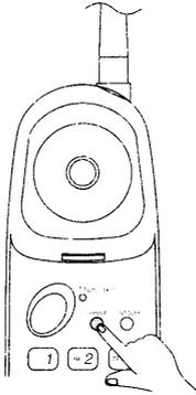
Your FT-6305 selects the channel by pressing the CHANNEL button when interference noise is heard. TALK/BATT. LED keeps lighting while Talk mode and Intercom mode.
