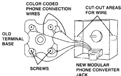
A modular jack converter (not included) is required, entailing some rewiring (namely, making color-coded connections).
