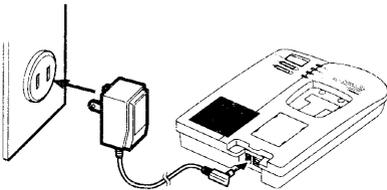
Connect the plug at the end of the AC adaptor to a standard 120V AC outlet and the other end to the rear of the base unit.
