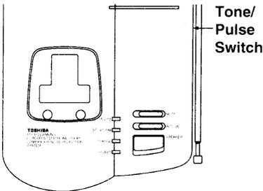
Set the TONE/PULSE switch located on the side of the base unit for the type of service you have (tone or pulse). If you are not sure which type of service you have, do this simple test.
