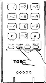
The FLASH button is used to send a timed hookflash on the telephone line for accessing services such as call waiting, etc. (Call Waiting is a telephone company service).
