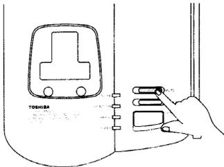
Pressing the MUTE button turns off the microphone during a telephone conversation at the speakerphone and the intercom so that you may speak to someone in the room with you without the caller overhearing. The SP/INTCOM LED will blink in this mute mode. Press the SPEAKERPHONE button or MUTE button again to resume normal conversation.
