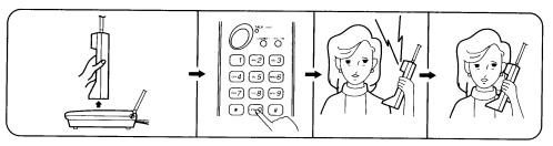
Lift the handset from the base unit, and press the TALK button. The TALK/BATT. LED lights.
