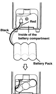
First, remove the battery compartment cover on the back of the handset by sliding it down.
