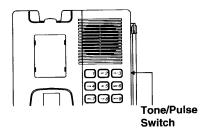
Set the TONE/PULSE switch located on the side of the base unit for the type of service you have (tone or pulse). If you are not sure which type of service you have, do this simple test.
