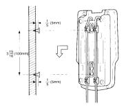
(3) Place the base unit on the screws and push down until it is firmly seated. Then connect the AC adaptor into a wall outlet.
