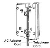
Place the base's keyhole slots over the two screws and gently push down on the base unit to lock it into place.
