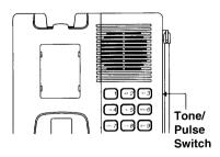
Set the TONE/PULSE switch located on the side of the base unit for the type of service you have (tone or pulse). If you are not sure which type of service you have, do this simple test.
