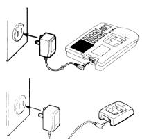
Connect the plug at the end of the AC adaptor to a standard 120V AC outlet and the other end to the rear of the base unit.
