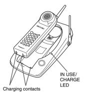
(5) Place the handset on the base unit. Be sure the IN USE/CHARGE LED lights. If the IN USE/CHARGE LED does not light, make sure the AC adaptor is plugged in securely and that the electrical outlet is working and not controlled by a light switch.
