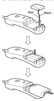
Use only the spplied battery pack (TRB-8000; power source 600 mAh. 3.6V).
