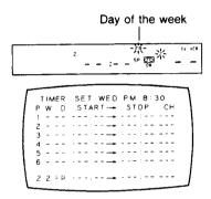
6 Set the desired hour of the recording "ON" time "PM 9" by pressing the *UP* or the *DOWN* button, and then press the *SET* button.
