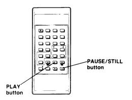
Press the PAUSE/STILL button during playback and keep the button pressed. Frames will be continuously advanced.
