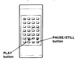
Press the PAUSE/STILL button during playback to freeze the picture.
