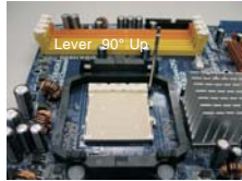
STEP 1: Lift Up The Socket Lever
