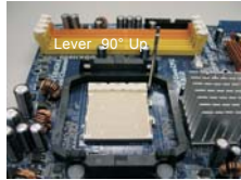
STEP 1: Lift Up The Socket Lever
