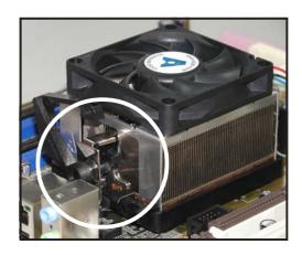
4. Push down the retention bracket lock on the retention mechanism to secure the heatsink and fan to the module base.
