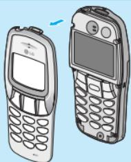
2. To replace the cover, first place and close the catch in the lower part of the cover into the corresponding hole in the phone and then gently close the whole cover.
