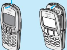
1. To remove the cover, press the locking catch of the cover for example with a coin, Start to open the cover from its upper part.
