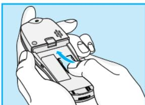
Locate the SIM card socket in the back of the phone.
