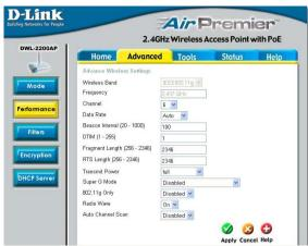
Beacon Interval- Beacons are packets sent by an access point to synchronize a network. Specify a beacon interval value.
