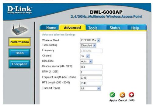
The **default** Performance settings are shown in the illustration above. **Wireless Band:** Select **802.11a** (up to 108 Mbps speed in turbo mode in the 5GHz range) or **802.11b** (up to 22 Mbps speed with AirPlus adapters.)
