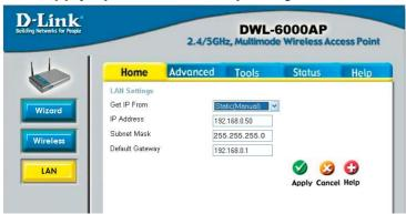
This window displays the default settings of the DWL-6000AP. The default IP Address is 192.168.0.50. If you select **Dynamic IP Address**, you will obtain a dynamic IP Address from a DHCP server on your network.
