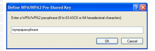
Enter a passphrase into the box as seen above. The passphrase is an alpha-numeric password between 8 and 63 characters long and can include symbols (!?\*&\_) and spaces. This passphrase must be exactly the same on all other wireless devices on your network. Click the **OK** button to save your settings.
