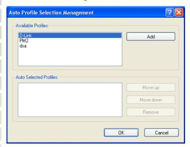
To add a profile to the Auto Selected Profiles list, highlight the profile and click **Add**. The Move Up and Move Down buttons will allow you to prioritize multiple profiles.
