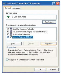
Input your **IP address and subnet mask**. (The IP addresses on your network must be within the same range. For example, if one computer has an IP address of 192.168.0.2, the other computers should have IP addresses that are sequential, like 192.168.0.3 and 192.168.0.4. The subnet mask must be the same for all the computers on the network.)
