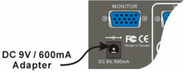
Step 9. Now power up all computers simultaneously. The first computer that is connected to port PC1 will be shown on the monitor. You may check to see if the mouse and keyboard work after the system has booted up. If this is OK, use the "Select" button to choose the next computer and verify the functionality in the same way. If you find errors, re-check all cables for proper connections before going to the troubleshooting section of this manual.
