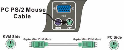
**Step 6**. To finish the hardware installation, connect the PS/2 keyboard cables from your computers to the DKVM-2/4 unit. Connect a keyboard cable (6-pin Mini DIN Male / Male) to the PC and to
