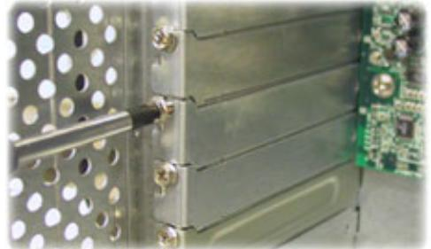
Locate an available PCI slot and insert the **DUB-A2** carefully into the PCI slot.
