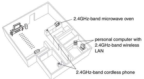
The surround speaker will automatically seek a clear channel if any of these other devices interfere with its communication. When this happens, the wireless link indicator ("W") flashes on the main unit, and there is a brief interruption in audio coming from the surround speaker.
