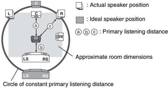
If either distance (a) or (b) is less than (c), find the difference in the table and change to the recommended setting.
