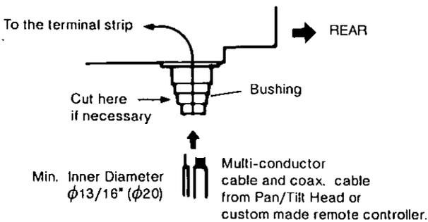
Pass the cables through the wiring hole.
