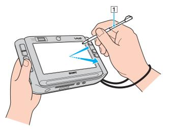
Take out the stylus from the back of your computer and use it for the following actions on the touch panel LCD screen, as well as handwritten entries. This stylus is extendable. Slide it out to its full length if necessary.
