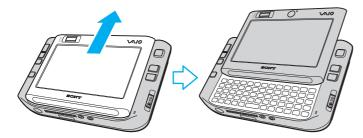
Keep your fingers off the screen surface while sliding up the touch panel LCD screen.
