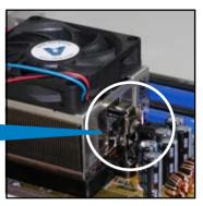
Align the other end of the retention bracket (near the retention bracket lock) to the retention module base.
