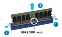
2. Remove the DIMM from the socket.
