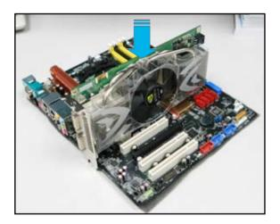
4. Insert the second graphics card into the other slot. Make sure that the card is properly seated on the slot.
