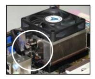
Push down the retention bracket lock on the retention mechanism to secure the heatsink and fan to the module base.
