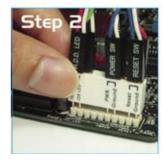
When installed, the Q-connector appears as shown.
