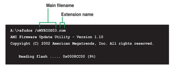
3. The utility will copy the current system BIOS by default to the floppy disk. Make sure that the floppy disk has at least 600KB of free disk space and is not write-protected.
