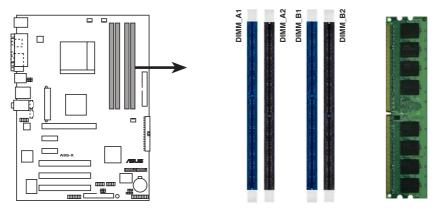
A8S-X 184-pin DDR DIMM sockets
