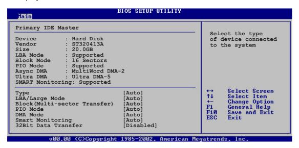
The values opposite the dimmed items (Device, Vendor, Size, LBA Mode, Block Mode, PIO Mode, Async DMA, Ultra DMA, and SMART monitoring) are auto-detected by BIOS and are not user-configurable. These items show N/A if no IDE device is installed in the system.
