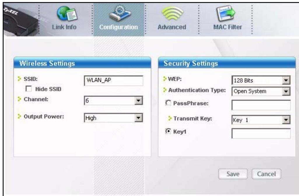
The screenshot displays the ZyXEL AG-120 Configuration screen. At the top, there is a navigation bar with four tabs: 'Link Info', 'Configuration' (which is highlighted), 'Advanced', and 'MAC Filter'. Below the navigation bar, the main content area is divided into two panels: 'Wireless Settings' and 'Security Settings'.
