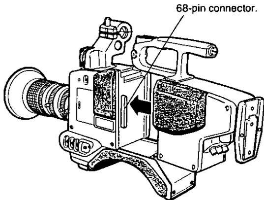
1-2 Tighten two Camera Adaptor Holding Screw/knob (2) firmly and make sure the adaptor is securely fixed to the camera.
