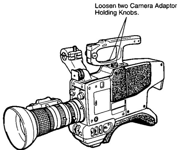
2-2 Remove the Camera Adaptor while pressing up the Release Button underneath the camera.
