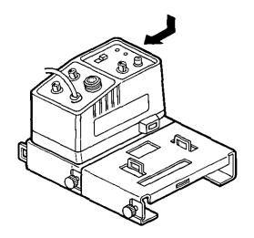
Note : When multi AC adaptors are used, the mounting bases can be attached as shown above.
