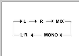
You can select the mode in which the sound is reproduced on the loudspeakers and AV outputs. The following options are available.
