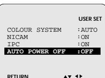
The Auto Power Off feature automatically turns off your DVD-VCR if no signal is received and you do not press any button for the selected time.
