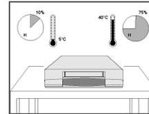
Do NOT expose the DVD-VCR to extreme temperature conditions (below 5°C and above 40°C) or to extreme humidity conditions (less than 10% and more than 75%).
