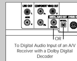
To Digital Audio Input of an A/V Receiver with a Dolby Digital Decoder
