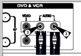
You can connect other audio/video equipment to your DVD-VCR using audio/video cables if the appropriate outputs are available on the equipment chosen.
