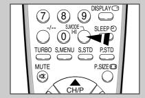
The "S.MODE I-II" button displays/controls the processing and output of the audio signal. When power is switched ON, the mode is automatically preset to either "Dual-I" or "STEREO", depending on the current transmission.
