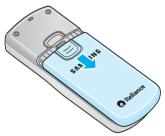
2. Place the battery into the battery slot, making sure that the metal contacts is facing down.
