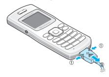
**Note**: Do not remove the battery from the phone without unplugging the adapter while it is charging. Otherwise, the phone may be damaged.
