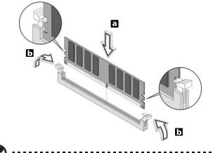
**Note:** The DDR2 DIMM sockets are slotted to ensure proper installation. If you insert a DDR2 DIMM but it does not fit easily into the socket, turn the DDR2 DIMM around and try to insert it again.
