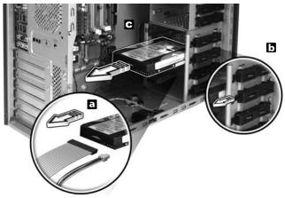
Insert the new hard disk into the frame (a).
