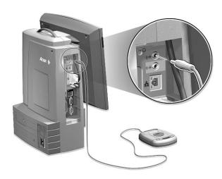
• other audio line-out devices: connect to the Line-out port (lime port) located on the left panel of your computer.
