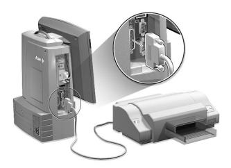
To connect a serial printer, plug the printer cable into the serial port [OO] (teal or turquoise port) located on the left panel of your computer. See "Left panel" on page 14 for the location of the serial port.
