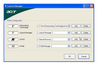
Launch Manager allows you to set the four easy-launch buttons located above the keyboard. "Easy-launch buttons" on page 27 for the location of the easy-launch buttons.
