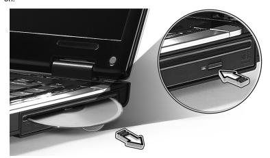
Insert a clip to the emergency eject hole to eject the optical drive tray when the computer is off.
