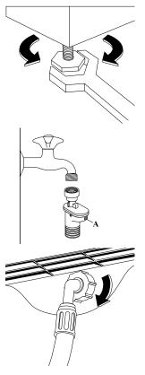
The inlet hose must not be lengthened. If it is too short and you do not wish to move the tap, you will have to purchase a new, longer hose specially designed for this type of use.
