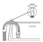
The end of the drain hose must always be **ventilated**, i.e. the inside diameter of the drain pipe must be larger than the outside diameter of the drain hose.
