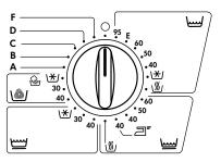
Position "E" corresponds to the ENERGY SAVING programme at approx. 67°C for normally soiled laundry, extended washing time (cannot be combined with 번 (QUICK).
