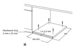
With the appliance installed adjust all four feet ensuring the machine is stable, and a clearance of approximately 5 mm is left between the top of the machine and the underside of the worktop.
