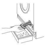
Place a container under the filter and unscrew it: sol
