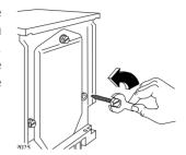
Remove the polystyrene base and take off the bottom panel by unscrewing the central screw.
