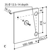
The required dimensions are given in the picture C.
