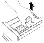
To remove the drawer from the machine, press the button in the rear left-hand corner.
