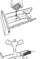
7. Use a brush to clean the entire compartment area of the washing machine, particularly also the nozzles on the top side of the compartment.
