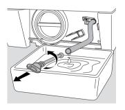
Discard the water from the container, replace it under the emergency emptying hose and remove the plug from the hose.
