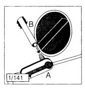
Allow the residual water to drain into a bowl (place a cloth underneath). Depending on the amount of residual water, it may be necessary, to empty the collecting bowl several times. **Take care when the suds are hot!** Where necessary, allow to cool first!
