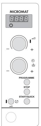
1. Press the START-button 'START/QUICK' three times. The time appears in the display and the programme begins. The microwave power signal lamp comes on.
