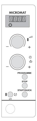
1. Press the button for automatic programmes '**PROGRAMME**' until the desired programme appears in the display.
