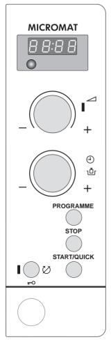
1. Plug the appliance into the mains. The display starts to flash «**AEG**» and then «**DD:DD**». The dots between the digits blink rapidly.
