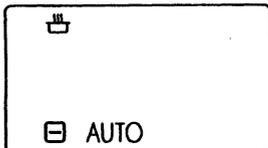
**4.** When the sensor detects the vapour and aroma emitted from the food, the remaining reheating time will appear on the display, and counts down in seconds.
