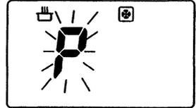
6. Touch **POWER LEVEL** pad to set power level for microwaving.
