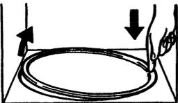
**A. Turntable Tray (glass)** — It rotates clockwise or anti-clockwise during cooking. To remove the turntable, push the rim down and lift out.
