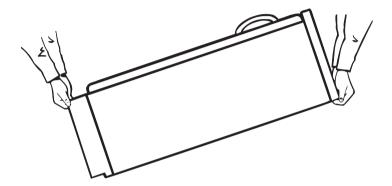
2. In order to push the appliance into its final position, press carefully at the top of the door and tip the appliance back slightly. The weight is then transferred to the back wheels and the appliance can be easily pushed.
