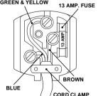
3.The wire coloured brown must be connected to the terminal marked "L" or coloured red.
