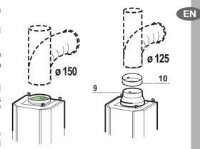
Before fitting the chimney to the canopy make the electrical connection as described in the section titled EN "ELECTRICAL CONNECTION".
