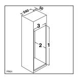
Fit the appliance in the niche by making sure that it stands against the interior surface of the unit on the opposite side where the door hinges of the appliances are fitted. Insert the appliance until the upper strip butts up against the unit (1) and make sure that the lower hinge is in line with the surface of the unit (2).
