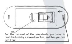
Lamp specification: 220 to 240 V, max 15W bulb holder: F14
