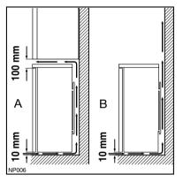
There should also be a gap of 25 mm either side of the appliance. Do not obstruct the space underneath. The back of the cabinet may be placed close to the wall but must not touch it. DO NOT install in places with restricted ventilation.
