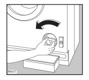
Unscrew and remove the filter.
