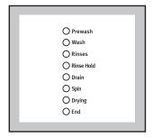
The "End" pilot light flashes in the event of operating problems and the corresponding alarm code appears on the display.
