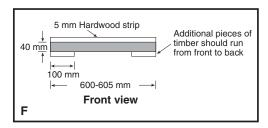
Drill four fixing holes see Fig. G
