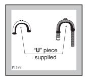
TPlace the drain hose into your standpipe, which should have an internal diameter of approximately 38mm thus ensuring there is an air break between the drain hose and standpipe.
