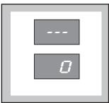
If the programme selector dial is on the Reset **Off** position, three flashing dashes will be displayed. If the programme selector dial has been left on a wash programme position at the end of the previous washing cycle, a flashing zero appears on the display.
