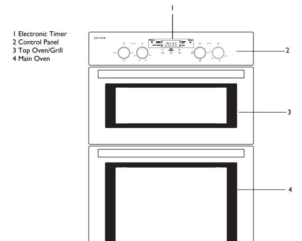
Your built-in oven comprises of a conventional top oven and dual grill in the top compartment. The main fan oven is the larger of the two ovens. It can be automatically controlled by the electronic timer.
