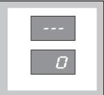
If the programme selector dial is on the "Off" (Reset) position, three flashing dashes will be displayed. If the programme selector dial is positioned on a wash programme, a flashing zero appears on the display.
