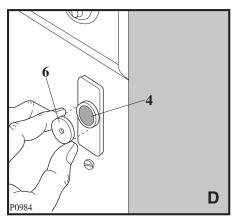
If the door has to be opened from left to right, invert the position of the plates (7), the magnet (4) and the plate (5) (Fig. B and E). Mount the countermagnet (6) and the hinges (1) as previously described.
