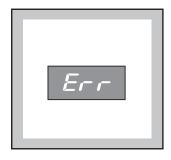
An alarm code indicates a fault in the machine operation (see page 29, "Something Not Working").
