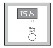
The delay time is displayed for 3 seconds, then the duration of the selected programme reappears. After you have pressed the **Start/Pause** button, the countdown is updated every hour, and, for the last two hours, every 30 minutes.
