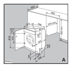
When installing the appliance into the kitchen furniture ensure, if possible, the hoses are placed in either of the two recesses on the back of the appliance. This will help to prevent the hoses from becoming kinked or trapped. Fig. AB.
