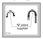
lace the drain hose into your standpipe, which should have an internal diameter of approximately 38mm thus ensuring there is an air break between the drain hose and standpipe.
