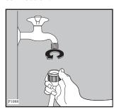
The inlet hose is provided with a water stop device, which protects against damage caused by water leaks in the hose which could develop due to natural ageing of the hose. This fault is shown by a red sector in the window "A". Should this occur, turn the water tap off and refer to your Service Centre to replace the hose.
