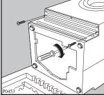
3 Repeat the operation for the left and central polythene bags. Re-fit the bottom panel using the 4 screws supplied with the door hinges (in the plastic bag) and the previously removed screw.
