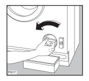
Unscrew and remove the filter.
