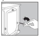
I Using a spanner unscrew and remove the rear right bolt. Lay the machine gently on its back, making sure that the hoses are not squashed.
