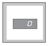
Delay start, a time value indicated in hours (23 hours max) and selected by means of the relevant button.
