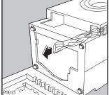
2 Remove the polystyrene base and take off the bottom panel by unscrewing the central screw. Carefully slide out the right polythene bag.
