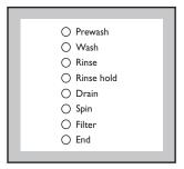
The "**End**" pilot light flashes in the event of operating problems. And the relative alarm code appears on the display.
