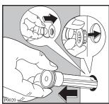
4 Set the machine upright and remove the two remaining bolts from the back.
