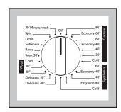
The selector dial can be turned either clockwise or anticlockwise to select the required wash programme .
