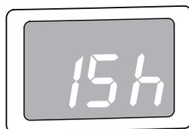
The delay time (20 hours max) is displayed for a few seconds, then the duration of the selected programme reappears.
